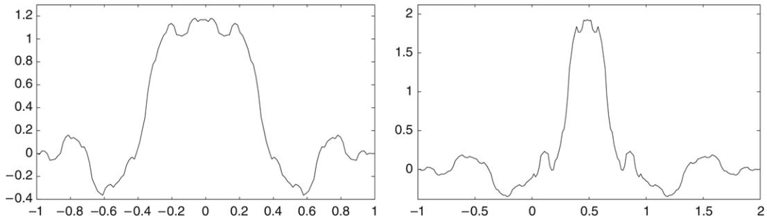
**Fig. 6.** The graphs of  $\tilde{\phi}_1$  (left) and  $\tilde{\phi}_2$  (right) in the symmetric dual 2-refinable function vector  $\tilde{\phi} = [\tilde{\phi}_1, \tilde{\phi}_2]^T$  constructed in Example 5.2 for the interpolating 2-refinable vector in Example 4.1. Moreover,  $v_2(\tilde{\phi}) \approx 1.117992$  and  $\tilde{\phi}_1(-x) = \tilde{\phi}_1(x)$  and  $\tilde{\phi}_2(1-x) = \tilde{\phi}_2(x)$  for all  $x \in \mathbb{R}$ .
