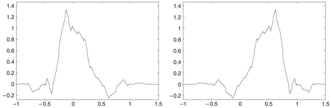
**Fig. 4.** The graphs of  $\phi_1$  (left) and  $\phi_2$  (right) in the orthogonal interpolating 3-refinable function vector  $\phi = [\phi_1, \phi_2]^T$  of Example 4.4. Moreover,  $\nu_2(\phi) \approx 1.046673$  and  $\phi_2(1/2 - x) = \phi_1(x)$  for all  $x \in \mathbb{R}$ .
