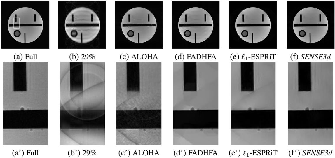
**Figure 4.** MRI Phantoms of Slice 1 with size 512-by-512. (a) Reference SoS image by four full  $K$ -space data with zoom-in area. (b) SoS image by four coil images by 29%  $K$ -space data on uniform sampling mode in Figure 3(a). (c) ALOHA. (d) FADHFA. (e)  $\ell_1$ -ESPIRiT. (f) Our proposed 3D-US model. (a')–(f') are the zoom-in parts of (a)–(f), respectively.
