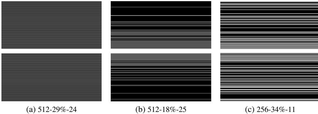
**Figure 3.** Sampling modes for the  $K$ -space. (a) 29% data by the uniform sampling model of  $512 \times 512$  (one line taken from every four lines) with 24 ACS lines (the middle white area); (b) 18% data by the random sampling model of  $512 \times 512$  with 25 ACS lines; (c) 34% data by the random sampling model of  $256 \times 256$  with 11 ACS lines.
