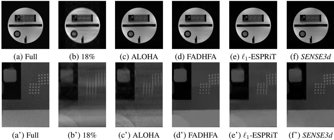
**Figure 5.** MRI Phantoms of Slice 2 with size 512-by-512. (a) Reference SoS image by four full  $K$ -space data, (b) SoS image by 18%  $K$ -space data with sampling model in Figure 3(b). (c) ALOHA. (d) FADHFA. (e)  $\ell_1$ -ESPIRiT. (f) Our proposed SENSE3d model. (a')–(f') are the Zoom-in parts of (a)–(f), respectively.
